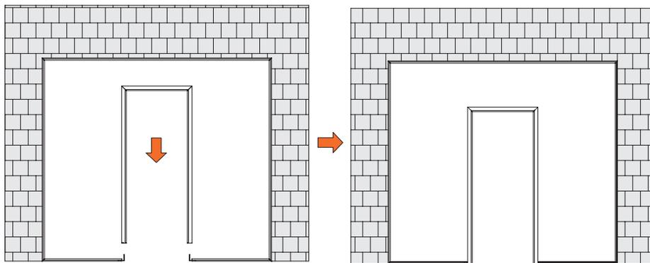
Insert the door intrados into the frames (previously screwed on the profix) and tighten the screws.
