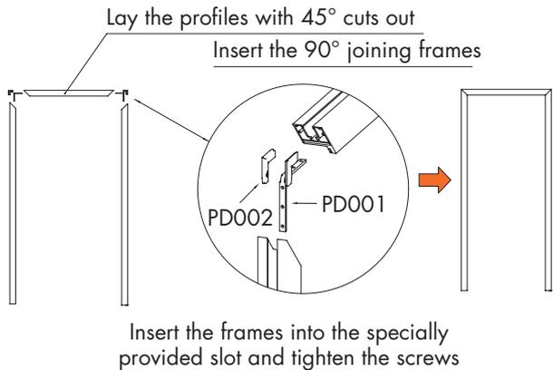
NOTE: make the Ø10 mm holes on the Profix profiles to tighten the frames' screws.
