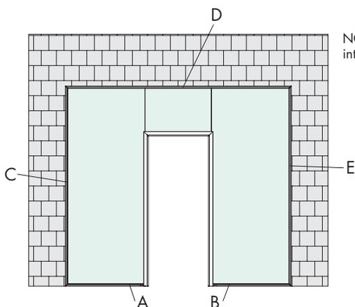
NOTE: for the Profix frontal closing profiles next to the intrados A and B, cut the flap as shown in the picture
