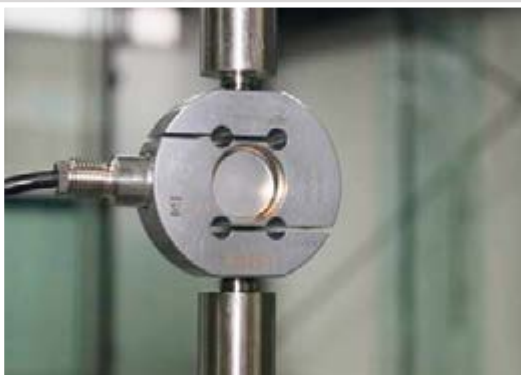
Load cell (maximum load: 2.0 kN)
