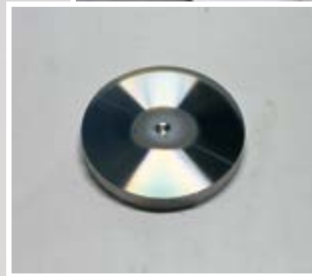
Bonding surface stressed after tests
