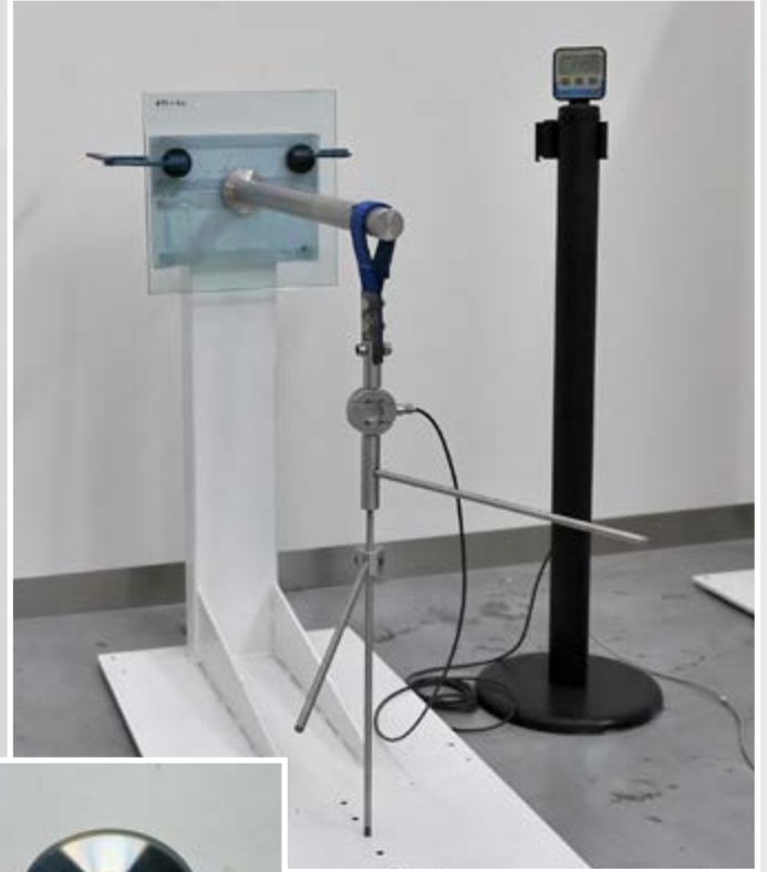
Tensile/shear strength resistance test steel disc \varnothing 75 mm
