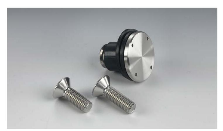
FIXING STUD Material: AISI 316 stainless steel With countersunk screws M12 x 30 mm, M12 x 35 mm, M12 x 40 mm Finish: //8 //15 Recommended installation tool Art. UT300
