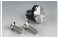
FIXING STUD Material: AISI 316 stainless steel With countersunk screws M12 x 30 mm, M12 x 35 mm, M12 x 40 mm. Compatible with bracket SB200ST. Recommended hole size Ø32 mm
