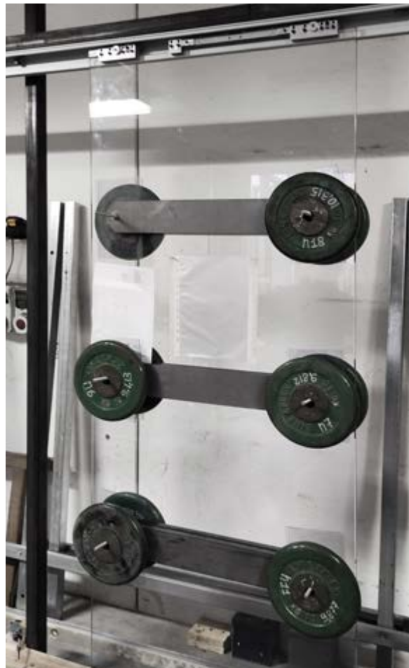
Test de surcharge
