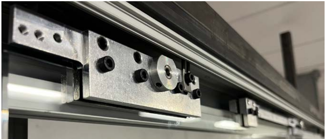
Clamp made entirely of aluminium
