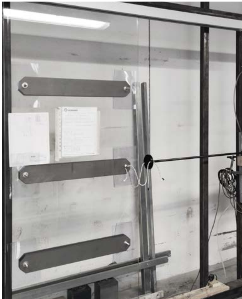
Tested performance of up to 45,000 opening and closing cycles
