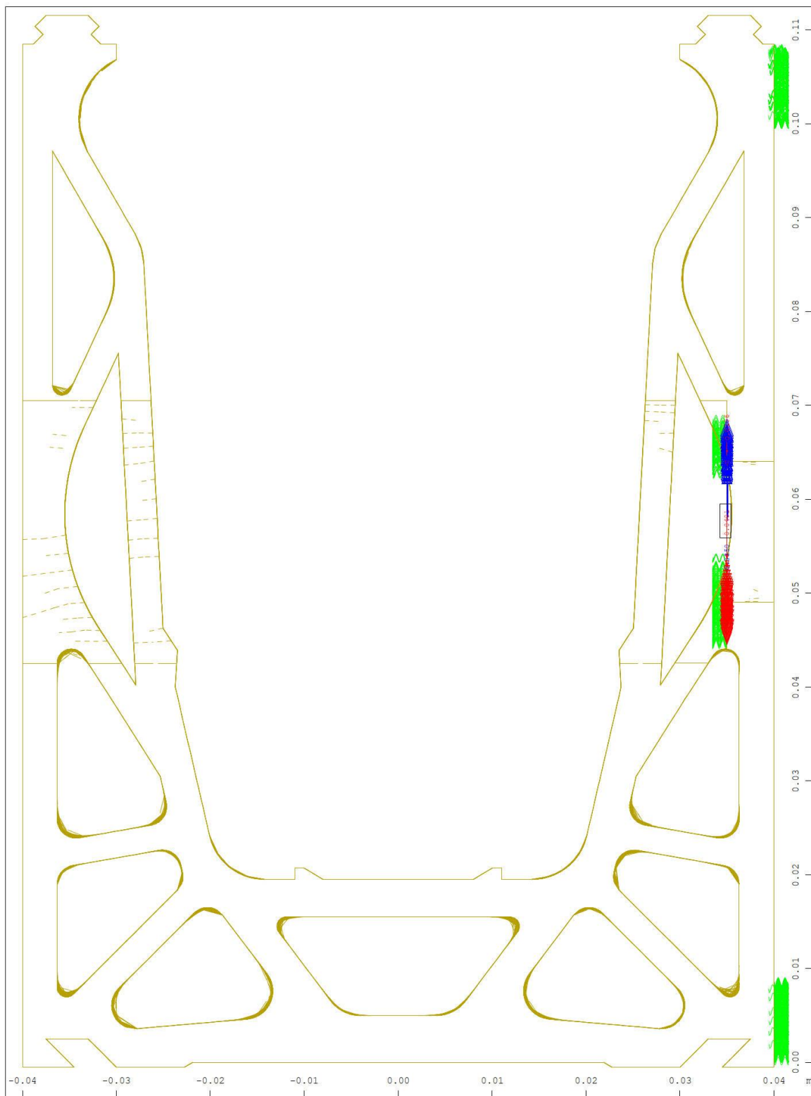
y Sector of system Group 1 4 10 11 20 M 10 : 4.81 z-x Supporting springs , Spring force in global Y, nonlinear Loadcase 10 ULS , 1 cm 3D = 0.0200 kN (Min=-0.0401) (Max=0.0376) (total: -1.1921e-06)
