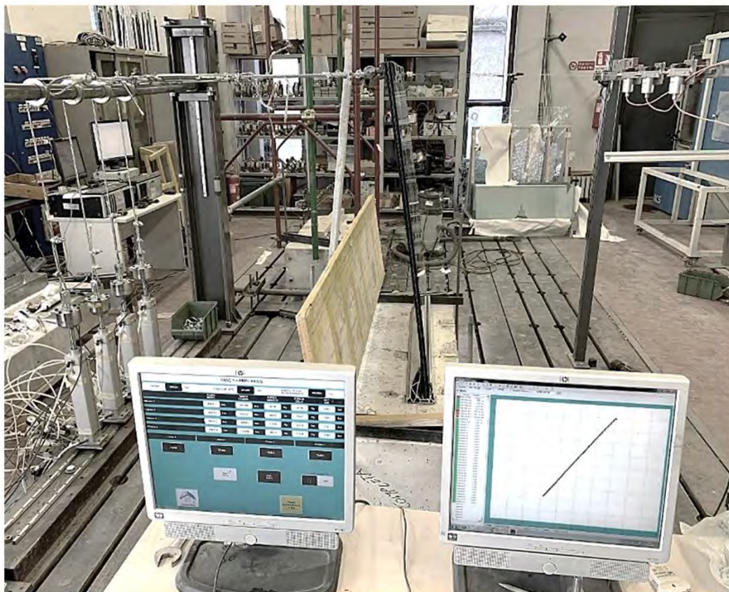
Figure 4.4 – Specimen snow: load application
