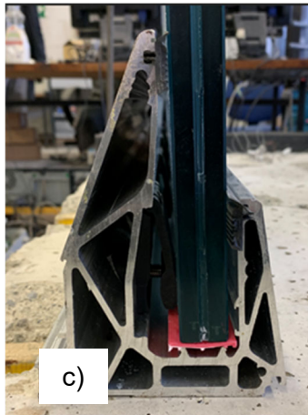
Figure 4.2 – Specimen WIND: load application and detail of failure
