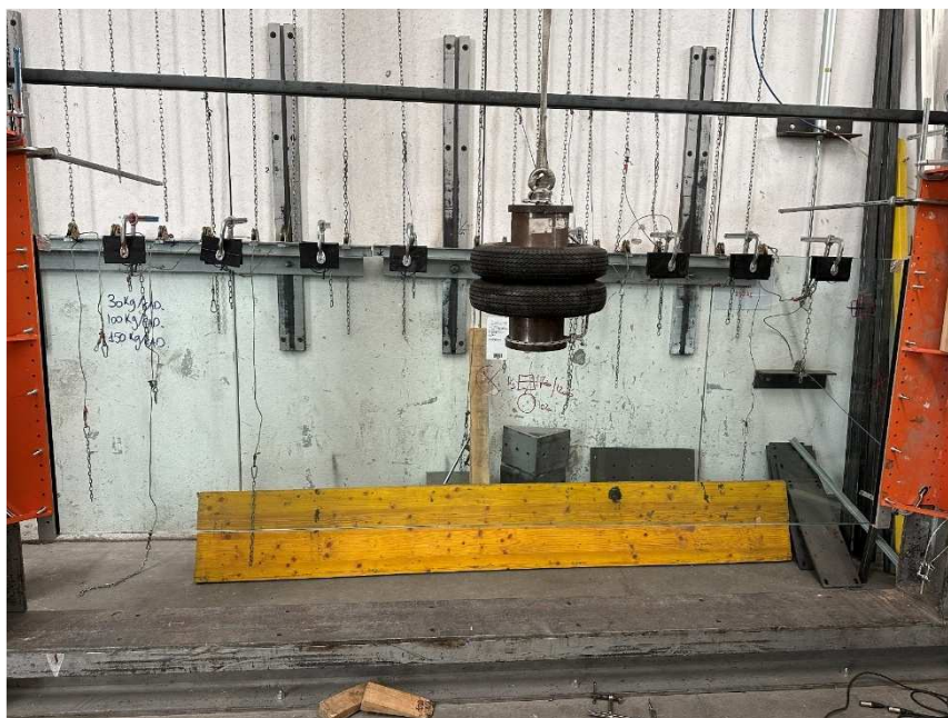
Photograph of the item after the impact 100 mm from the top edge
