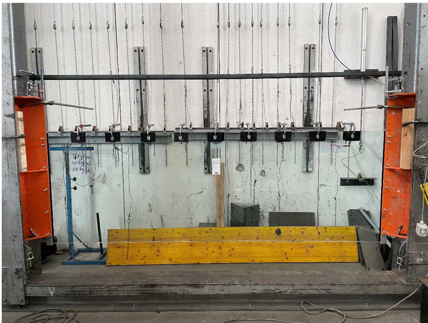
Photograph of the item secured to the test rig by a pair of steel supports for the two lateral aluminum profiles
