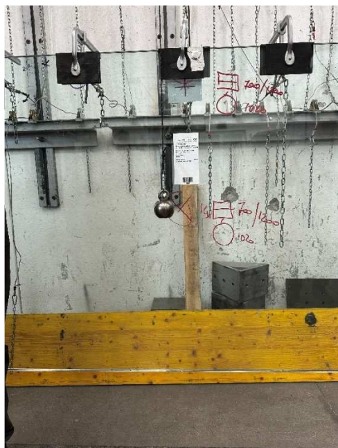
Photograph of the item after the hard body impact at the center of the infill
